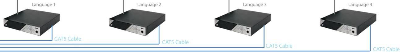
\*Transmitters to be placed closest to audience area for best transmission coverage \* ANT005 antennas can use WCA008 15m coaxial extension cables for longer reach.
